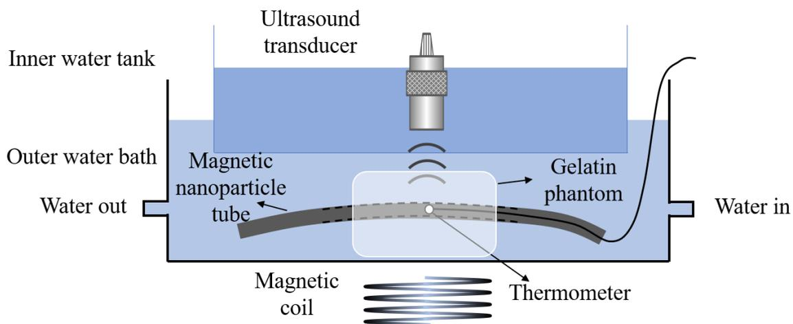
**Figure 3.** Experimental setup of the magnetically mediated thermoacoustic temperature measurement.
