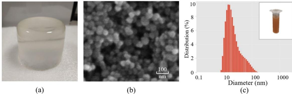
**Figure 2.** (a) Photograph of the prepared gelatin phantom, in which a magnetic nanoparticles tube is inserted. (b) Transmission electron microscopic image of the magnetic nanoparticles. (c) Size distribution of the magnetic nanoparticles.
