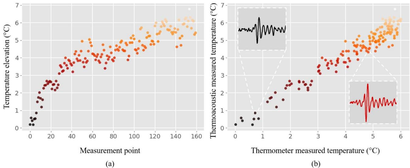
**Figure 4.** Magnetically mediated thermoacoustic temperature measurement results. (a) Temperature variation as hot water is gradually pumped into the water bath. (b) The relationship between the thermoacoustically measured temperature and the thermometer measured temperature. The insets show the thermoacoustic waveforms at two different measurement points.
