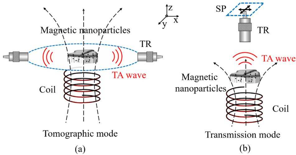
**Figure 1.** Two typical mode of magnetically mediated thermoacoustic detection: (a) tomographic mode; (b) transmission mode. Transducer: TR, thermoacoustic: TA, scanning plane: SP.
